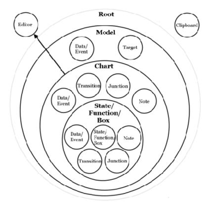
Rules of containment define the Stateflow hierarchy and the Stateflow API object hierarchy. For example, charts can contain states but states cannot contain charts. The hierarchy of Stateflow objects appears in the section "Stateflow Hierarchy of Objects" in the Stateflow and Stateflow<sup>®</sup> Coder<sup>™</sup> User's Guide. The Stateflow API hierarchy consists of these layers of containment:
