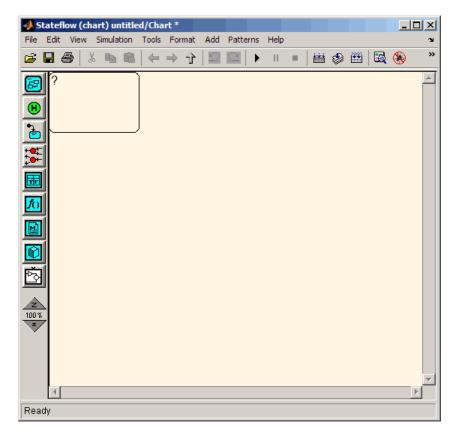
The constructor returns a handle to an API object for the newly created Stateflow object. Use this handle to display or change the object through its properties and methods.
