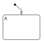
This method is also used for adding the default transitions toward the end of the example Stateflow chart constructed in "Creating New Objects in the Chart" on page 1-9.
