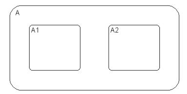
**5** Create a transition from the 3 o'clock position (right side) of state A1 to the 9 o'clock position (left side) of state A2 with these commands:
