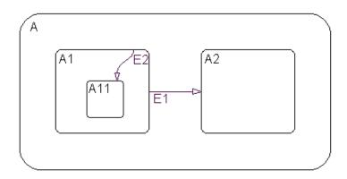
Both the state and transition labels in our example are simple one-line labels. To enter more complex multiline labels, see "Entering Multiline Labels" on page 1-38. Labels for transitions also have a LabelPosition property you can use to move the labels to better locations.
